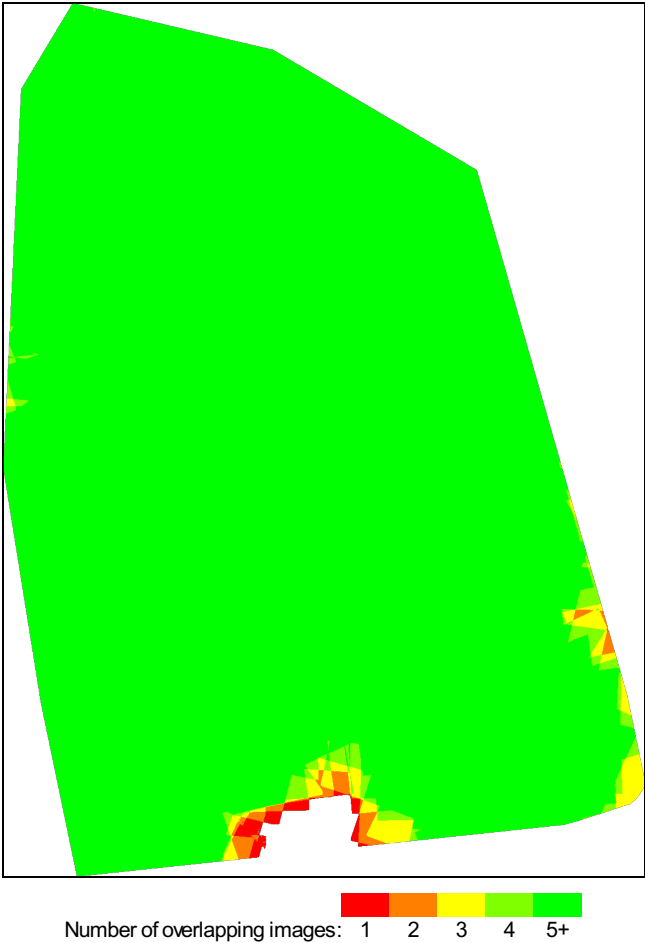
Figure 4: Number of overlapping images computed for each pixel of the orthomosaic. Red and yellow areas indicate low overlap for which poor results may be generated. Green areas indicate an overlap of over 5 images for every pixel. Good quality results will be generated as long as the number of keypoint matches is also sufficient for these areas (see Figure 5 for keypoint matches).
